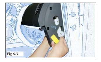
(d) Insert the V4 RES ECU Mounting Plate through the Hole on the side of the Dash. (Fig. 6-3)
