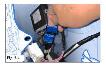
(f) Remove the Connector Block from the Vehicle's 22P Connector. (Fig. 5-4)
