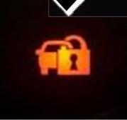
Security LED Turns ON solid for 30 Seconds then starts blinking
