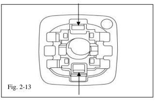
(j) Remove both driver side and passenger side visor clip bases by pressing in on the two inner tabs. (Fig. 2-13)
