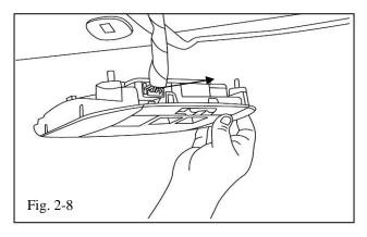
(3) Disconnect overhead console connector. (Fig. 2-8)
