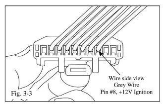
(c) Locate the GREY wire in pin #8 on the 10 pin connector. (Fig. 3-3)
