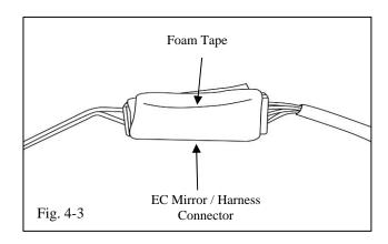
(c) Wrap one (1) piece of foam tape around EC mirror connector and EC harness connector. (Fig. 4-3)
