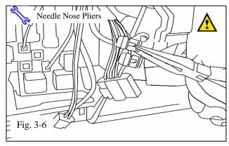
(f) Attach T-tap connector to WHITE/BLACK wire (pin #7) on the 10 pin connector with needle-nose pliers about 1.5 inches from the connector. (Fig. 3-6)
