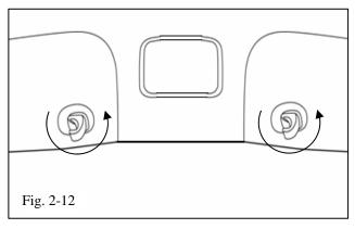
(i) Remove both driver side and passenger side sun visor clips by rotating counter clockwise. (Fig. 2-12)
