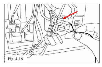
(q) Plug the BLACK wire spade end of the EC mirror harness into T-tap connector on the WHITE/BLACK wire. (Fig. 4-16)
