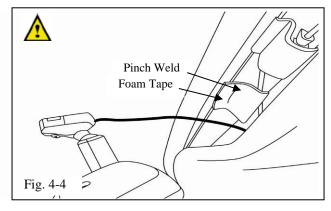
(d) Apply one (1) piece of foam tape to the pinch weld between the windshield and the headliner above the center of the mirror. (Fig. 4-4)
