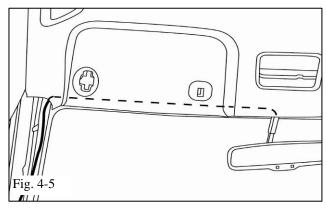
(e) Route the wire along the bottom curve of the headliner toward the A-pillar. (Fig. 4-5)
