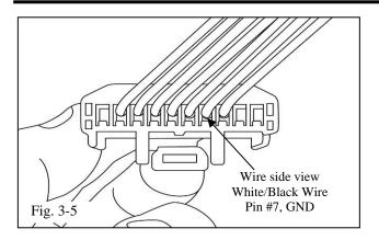
(e) Locate the WHITE/BLACK wire in pin #7 on the 10 pin connector. (Fig. 3-5)
