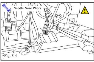
(d) Attach T-tap connector to GREY wire (pin #8) on the 10 pin connector with needlenose pliers about 1 inch from the connector. (Fig. 3-4)
