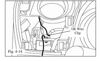
(o) Secure the EC mirror harness to the OE wire clip. (Fig. 4-14)
