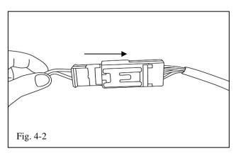
(b) Plug EC wire harness 2-pin connector into the 2-pin mirror harness. (Fig. 4-2)
