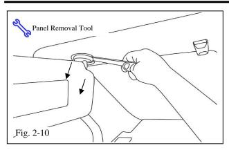
(g) Using panel removal tool, pry downward on visor mount to disengage two (2) clips. (Fig. 2-10)
