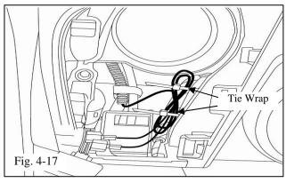
(r) Bundle any access wire and secure it to the OE harness with two (2) tie wraps. (Fig. 4-17)
