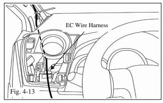
(n) Carefully route the harness through the dash panel to the front of the upper vent panel opening. (Fig. 4-13)
