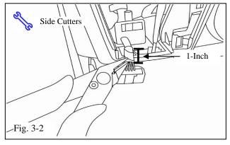
(b) Cut back approximately 1 inch of plastic tubing on the 10-pin connector wire bundle. (Fig. 3-2)
