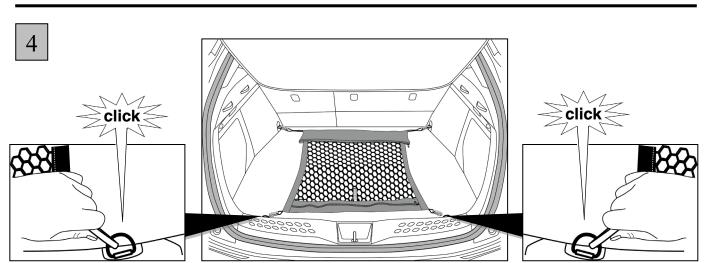
Tab to be rotated 90 degrees before placing in storage pouch.
