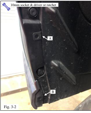
(b) Install supplied spring clips at locations A and B so that the factory divots are centers in the clips (Fig. 3-2).
