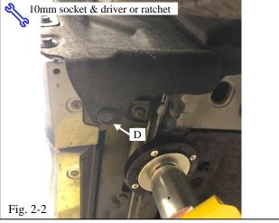
(b) Remove and save the pin in location D (Fig. 2-2).
