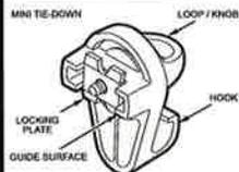
The bed rail system enables you to insert and move the mini tie-down to the best location along the bed rail to secure a load.
