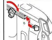
Tighten loop/knob in a clockwise motion until tight. Re-install end cap. Check tie-down to ensure that it is locked into detent and secure on rail.
