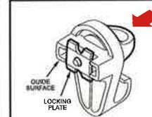
Depress the loop/knob so locking plate is equal with guide surface of the mini tie-down.
