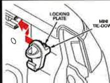
With the loop/knob depressed, slide the tie-down into the rail. Release the loop/knob once the tie-down enters the rail.
