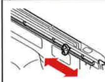
Slide mini tie-down to nearest detent position and snap into place. To move to another detent position, depress loop/knob to slide to next detent.
