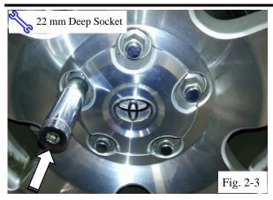
(c) Place the 22mm Deep Socket on top of the key. (Fig 2-3)
