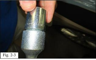
(c) Place the 21mm deep socket on top of the key (Fig. 2-3 & Fig. 2-4).
