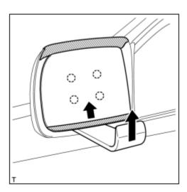
(b) Using a moulding remover, push the bottom of the glass upwards as shown in the illustration. Slide the glass upwards to detach the 4 claws, and remove the glass.
