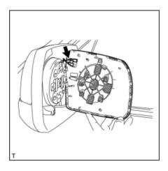
(c) w/ Mirror Heater: Disconnect the 2 connectors and remove the mirror glass.
