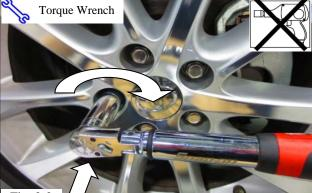
(c) Place the socket on top of the key. Apply pressure on the key, and using a torque wrench, tighten the wheel locks to 76 lbf•ft. (103 N•m). (Fig. 2-2).
