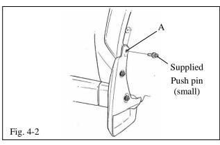
(b) Install supplied push pin (small) in location A while holding part up and into body panel (Fig. 4-2).
