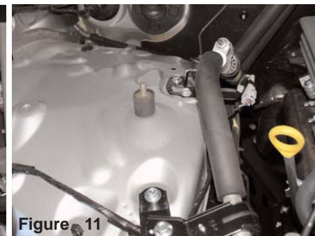
Figure 11 Screw the 8mm vibra-mount into the wheel well mounting location until the vibra-mount is sitting snug and flush over the mounting point.
