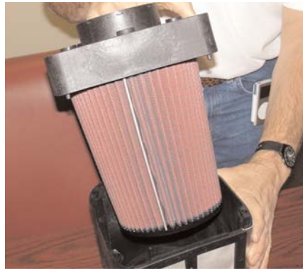
Once the screws have been removed, gently pull the base out of the Power-box body.
