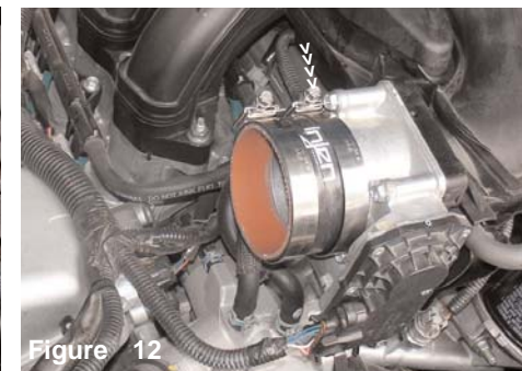
Figure 12 Press the 3" straight hose over the throttle body. Once the hose has been fitted over the throttle body, continue to use two power bands over the hose and tighten the band located over the throttle body.
