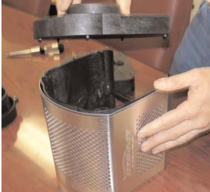
Once the screws have been removed separate the top stabilizer from the Power-Box body.
