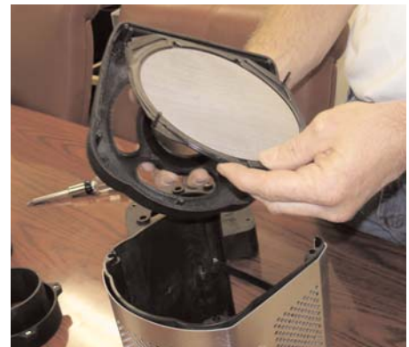
The round pre-filter screen will now detach itself from the stabilizer top for cleaning.
