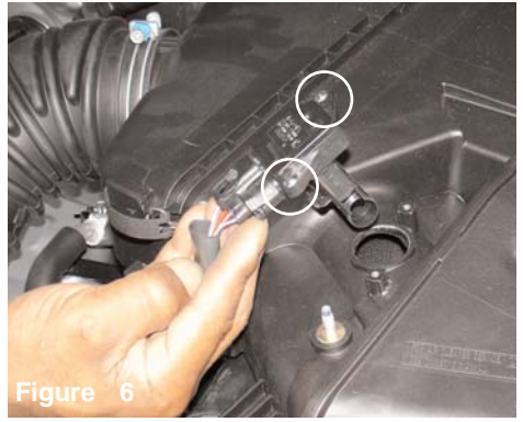
Figure 6 Unscrew the two screws from the mass air flow sensor, continue to remove the mass air flow sensor from the air box cleaner.
