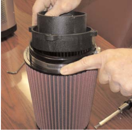
Once the clamp has been loosened, gently separate the velocity stack from the filter neck.
