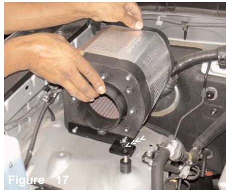
Figure 14 Align the power box bracket to the holes located on the base. Use the same m6 x 65mm bolts to fasten the bracket to the base.
