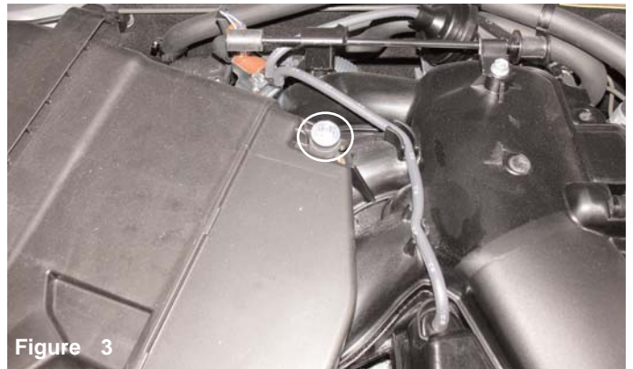
Figure 3 Unbolt the second m6 bolt located on the top of the air box cleaner as shown above. Removing these two bolt shown in figures one and two will allow you to remove the entire air box cleaner.
