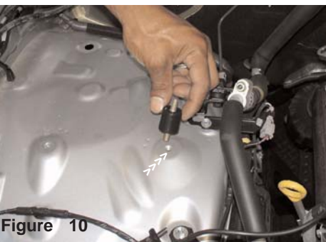
Figure 10 align the m8 vibra-mount to the pre-tapped hole located over the wheel well. It may be necessary to use a punch to drive a hole through the plastic liner underneath when installing the m8 vibra-mount.
