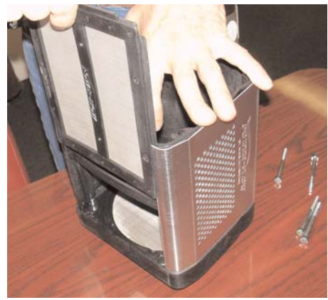
With the velocity stack base out of the way, the rectangular pre-filter screen will now slide out of the Power-box channel.
