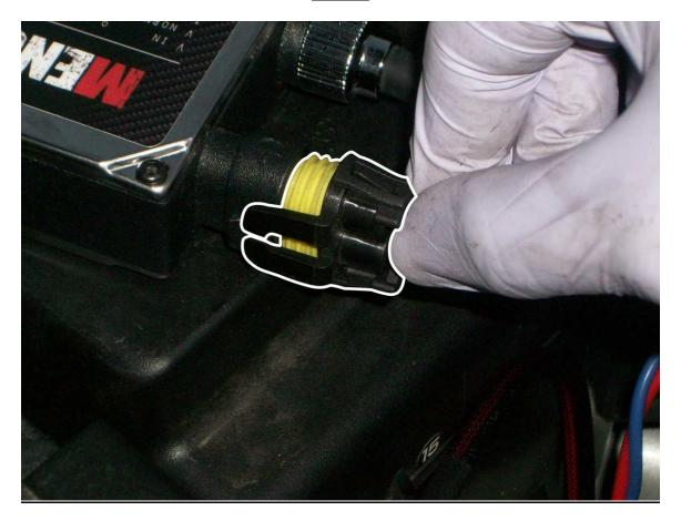
Performing <u>Step 8</u> will leave that ballast with an empty slot. Plug that female end with the male ballast plug from the relay harness. Relay harness wires may not be Red and Black, but instead Blue and Black or White and Black. Black will always be negative so ensure the positive wire is facing the positive (+) side of the ballast.
