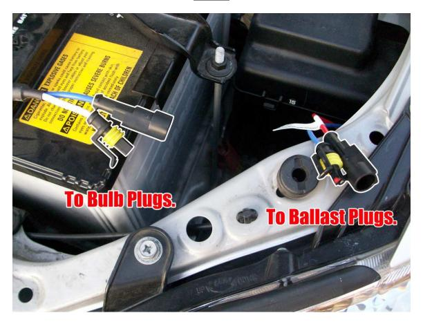
Locate the two HID bulb wires extending out of the base of the bulb. These two plugs will connect into the two similar plugs on the ballast. Each plug will distinctively connect into the other wire. Before connecting, it is a good idea to find a ideal spot to mount the ballasts. We include both double sided tape and ballast brackets to allow users on how to mount their ballasts. Please choose a smooth and safe location to ensure ballast reliability.
