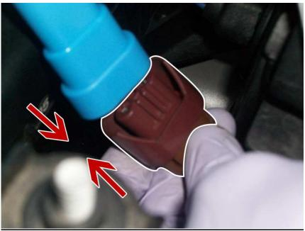
Both ends of the plug-and-play wire should fit as snug as possible to prevent them from coming lose during operation. Ensure the red wire of the plug-andplay wire is facing the positive (+) side of the ballast. Most vehicles cannot run their headlights if the plugs are in reverse polarity.
