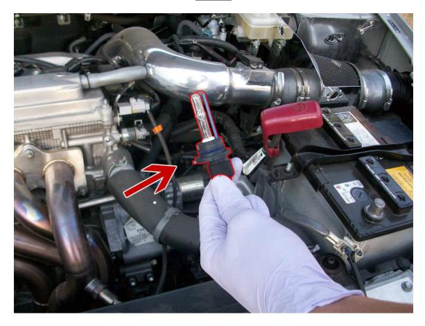
Grab one HID bulb by its base and insert into the empty headlamp socket. Once bulb is in place, turn the bulb by its base clockwise to lock the bulb back in place. Ensure the bulb is snug and is not loose.
