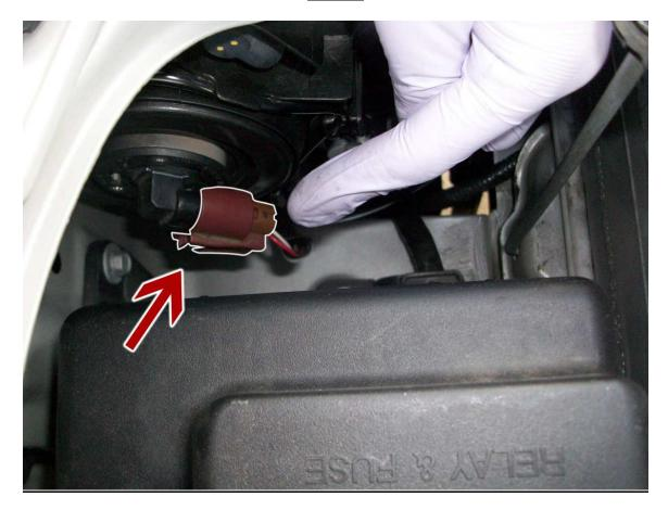
Locate the factory headlamp plug that is connected to the existing headlamp bulb. Press in the clip and remove the headlamp plug carefully. Once the plug is removed, turn the base of the bulb counter clockwise to unlock the bulb. Remove bulb and preserve in a safe place in case of future use.
