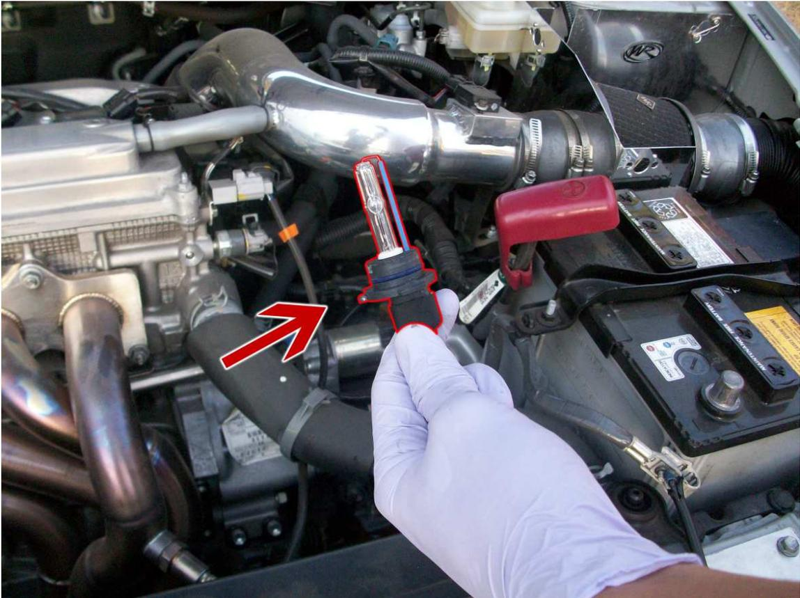
Grab one HID bulb by its base and insert into the empty headlamp socket. Once bulb is in place, turn the bulb by its base clockwise to lock the bulb back in place. Ensure the bulb is snug and is not loose.
