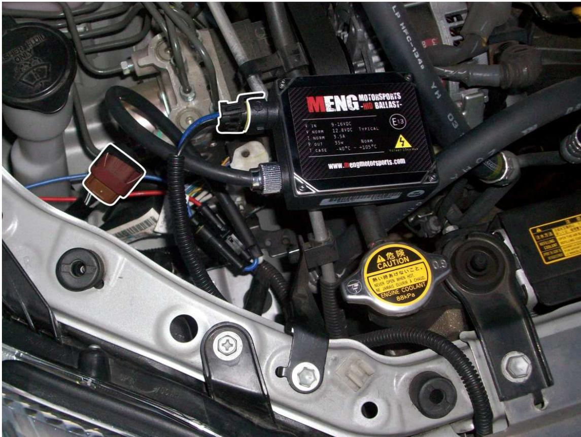
Now lets work on the other headlamp. Remove the plug-and-play wire from the other ballast and headlamp plug. By installing a relay harness, this plug-and-play wire will no longer be used. Tape off the factory headlamp plug to protect it from any debris. Connect the longer ballast plug into the ballast.
