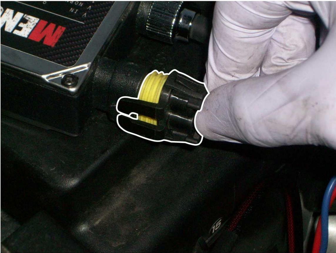
Performing Step 8 will leave that ballast with an empty slot. Plug that female end with the male ballast plug from the relay harness. Relay harness wires may not be Red and Black, but instead Blue and Black or White and Black. Black will always be negative so ensure the positive wire is facing the positive (+) side of the ballast.
