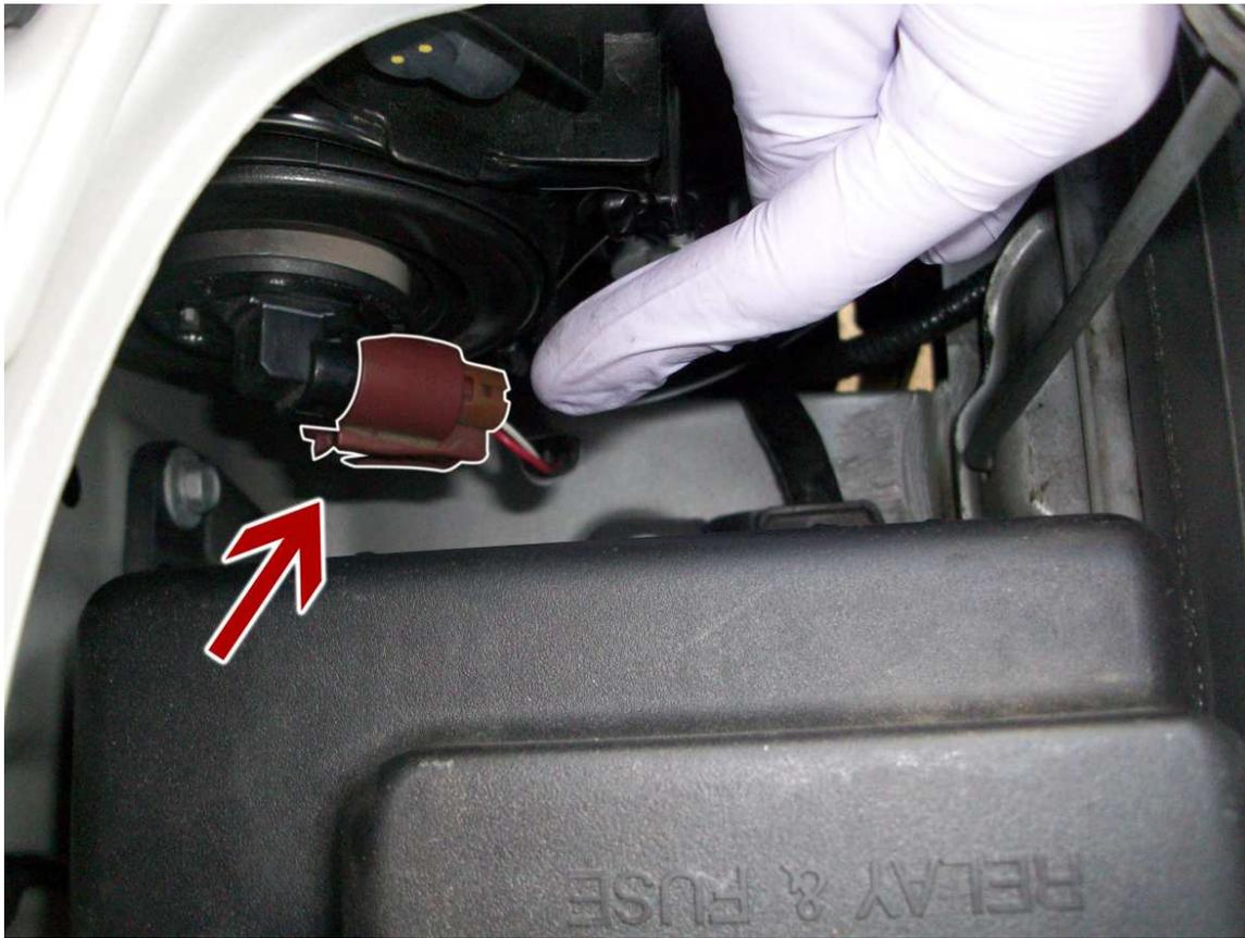
Locate the factory headlamp plug that is connected to the existing headlamp bulb. Press in the clip and remove the headlamp plug carefully. Once the plug is removed, turn the base of the bulb counter clockwise to unlock the bulb. Remove bulb and preserve in a safe place in case of future use.
