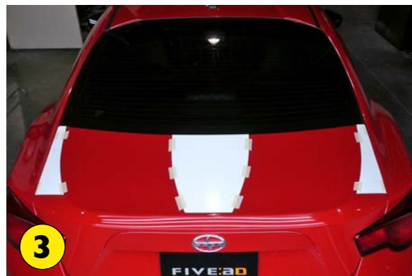
Templates Properly Located
