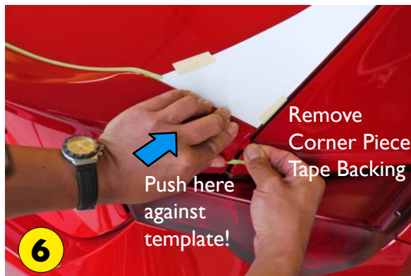
Adhering End of Spoiler to Decklid.
