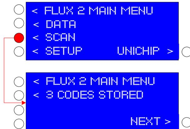
a. The display initially reports the number of Stored PID codes detected during the scan... in this example, the vehicle has three stored codes. To display the Stored PID codes, select the button left of the < 3 CODES STORED graphic.
