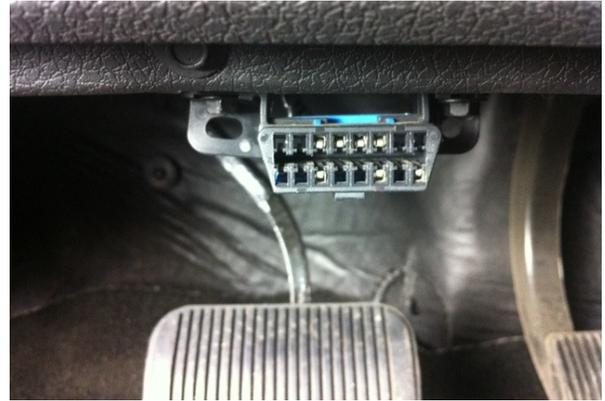
(2) By regulation, the OBD2 port will be located within two feet (61 cm) of the steering wheel and you will not need tools to access the port.
