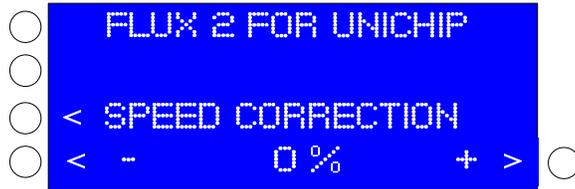
\*\*\* Note: The corrected speed reading is only in the Flux2 Display and the OEM speedometer is not affected.
