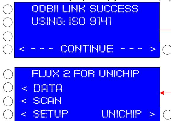
b. Once communication with the factory computer is established, the Flux2 display will automatically change to a Link Success display which confirms the OBD2 protocol in use. After 5 seconds the display will automatically advance to the Flux2 Main Menu Page. You may also press the buttons on either side of the **<--- CONTINUE --->** display to advance without any delay.
