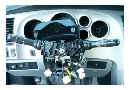
Now for one of the final parts...you need to remove the stalk assembly. You do this by using your needle nose pliers and punch the metal clamp. AT THE SAME TIME, you need to pull up the tab that is sticking straight up and pull the assembly towards you. It may be a little difficult to get loose. This is what it'll look like when removed:
