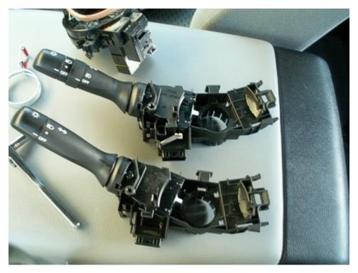
That's pretty much it. You need to install in the reverse order to get it put back together. Make sure when connecting the airbag back together you push the yellow clips in AFTER you have the connectors firmly seated in the panel.
