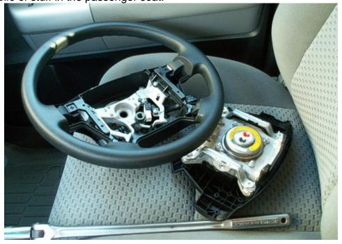
Take this time to remove the column shroud. You do this by pushing gently inwards; the top piece and bottom piece should separate. Be careful with the top piece, and you can pull the bottom piece out.
