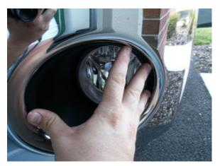
Now place the fog light into the black plastic housing. You will see how the housing is supposed to be inserted. When installing the fog light into the housing, make sure that the alignment screw will be on the bottom when placing it into the bumper (I think it's the only way it'll fit, too). It should snap into place.
