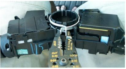
Once this is out, you need to push on the wipe stalk tab (circled in red). This will allow the wiper stalk to slide out. Place the wiper stalk back into the new assembly.
