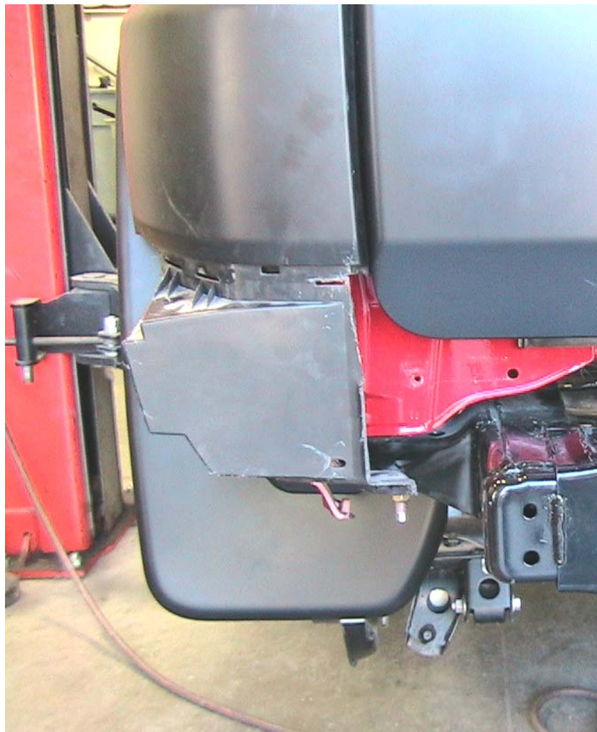
Figure 14 Rear view after final trimming, installed-LH
