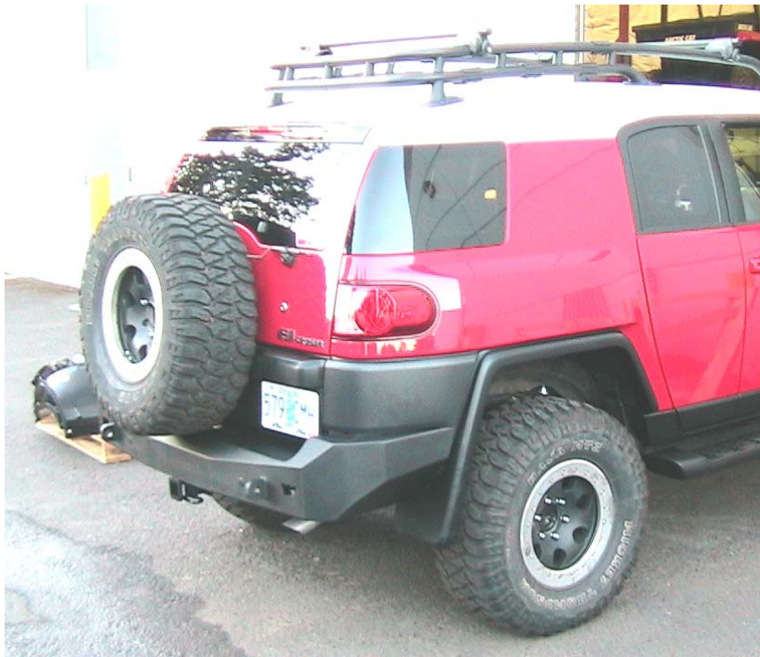
Figure 17 Bumper installation complete
