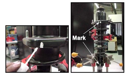
13) Carefully clamp the spring with your spring compressor and remove the plastic cap to expose the shaft nut. Remove the shaft nut using a 17mm socket.
