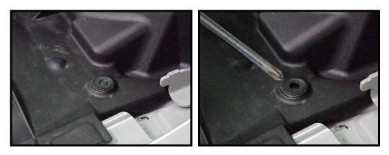
5) Spanning across the cowl panel is a rubber weather stripping which also clips into the cowl framing on each end and in the center of the panel. Carefully pop out each clip by using a needle nose pliers from underneath the cowl framing.
