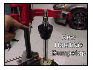
15) Make sure to keep the stock rubber seat for the lower perch. Also confirm that the rubber seat is oriented to match the lower perch.
