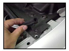
This document was created by Print2PDF http://www.software602.com 6) You should be able to remove the cowl panel by pulling forward. Now we can start removing the struts.
