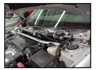
7) Remove the brake line/ABS bracket bolt using a 12mm socket. The ABS bracket should detach from the strut housing at this point.
