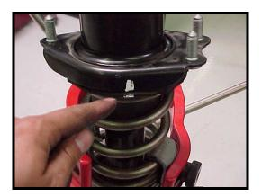
18) Install the washer and shaft nut onto the shaft and fully tighten the nut. Once the nut is tightened, carefully decompress the spring and make sure the top of the coil sits properly on the rubber boot seat. Don't forget to pop the plastic cap on the top.
