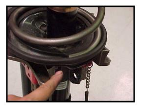
17) The rubber boot and the upper spring perch both have offset centers, so you will need to orient these correctly. The rubber boot has a small tab indicated in the picture. The upper spring perch has a cut out section in a similar fashion. When installed the tab will sit inside the cut out section and they will both be facing towards the spindle bracket mount on the strut.
