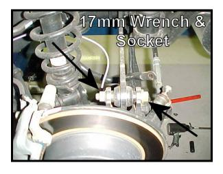
This document was created by Print2PDF http://www.software602.com 4) Remove the nut and bolt that secures the bottom of the shock to the lower control arm using a 19mm wrench and socket. At this point, everything under the fender should be detached from the shock.
