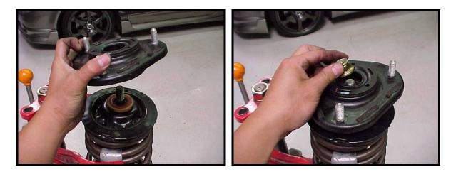
19) Slowly decompress the spring, making sure the top of the coil sits properly on the rubber seat of the boot. Don't forget to pop on the rubber cap over the shaft nut.
