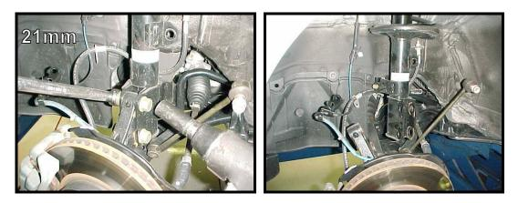
10) The only thing holding the strut to the car should be the 3 strut tower bolts. Loosen and remove each nut one at a time using a 14mm deep socket. When removing the last nut, reach down underneath the fender and hold onto the strut to keep it from falling.
