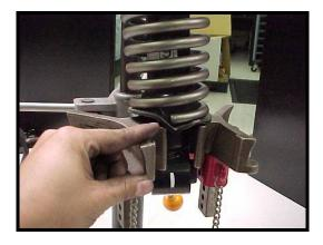
16) Notice the stock bumpstop is attached to a retaining washer, which needs to be reused with the included polyurethane bushing. Once attached, place the new bushing on the shock shaft.
