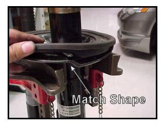
This document was created by Print2PDF http://www.software602.com 16) Place your new Hotchkis coil spring onto your strut as shown below. Again, safely clamp down the spring to install the remaining hardware.
