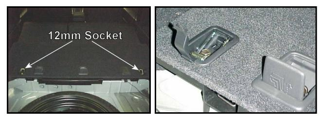
9) The plastic piece located underneath the panel you just removed will detach from the car by simply pulling it up.
