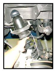
12) Before you remove the spring, you will need to mark the orientation of the upper spring perch relative to the shock body. Do this by using a paint marker or white out. Also try to mark the rubber boot seat as well.
