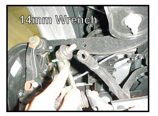
3) Next, remove the nut and bolt that secures the upper control arm to the rear spindle using a 17mm wrench and socket.
