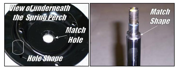
18) Next, place the upper mount plate on the shaft and secure it with the shaft nut. Fully tighten the shaft nut at this time.
