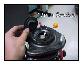
Tip: If at all possible, try to use an impact wrench to loosen the shaft nut.
