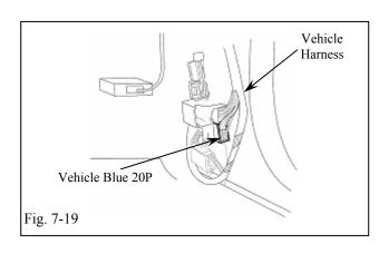
(x) Disconnect the Vehicle Harness' Blue 20P Connector. (Fig. 7-19)
