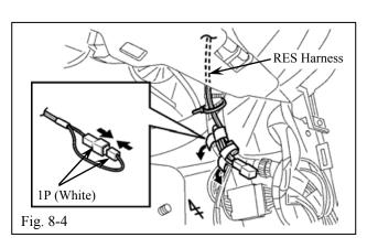
(e) Locate and disconnect the tape securing the V4 harness' white 1P RES Diagnostic Connectors from the Passenger side cowl area and connect them. (Fig. 8-4)
