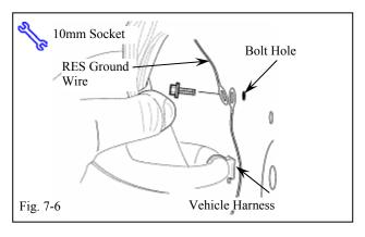
(g) Place the V4 Harness' Ground on top of the Vehicle's Ground. Re-install the Bolt back into the hole. (Fig. 7-6)
