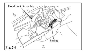
(f) Remove the Spring from the Hood lock assembly. (Fig. 2-6)
