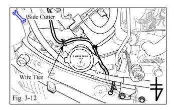
(n) Route the Hood Switch Harness towards the Firewall. Secure the Harness to the Vehicle Harness with 1 Wire Tie. (Fig. 3-12)
