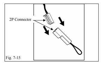
(q) Disconnect the V4 Harness' White 2P Connector.(Fig. 7-15)
