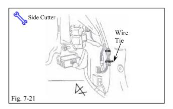
(z) Secure the 20P Connector with 1 Wire Tie as shown. (Fig. 7-21)
