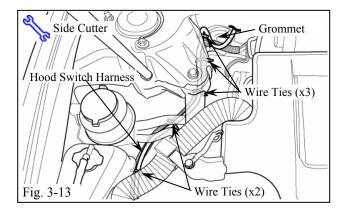
(o) Locate the grommet in the Passenger side engine compartment area. Route the Hood Switch Harness towards the Grommet securing it with 5 Wire Ties. (Fig. 3-13)
