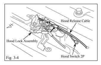
(e) Refit the Hood release cable to the Hood lock assembly. (Fig. 3-4)
