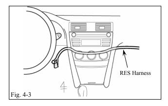
(g) Route the portion of the V4 Harness with the Relay, Fuse, and 8P White Connector through the Center Console to the Driver's Side. (Fig. 4-3)
