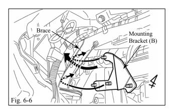
(g) Remove the Protective Sheet from the Butyl Tape. Insert the ECU Mounting Bracket (B) up behind the Vehicle Brace as shown.
