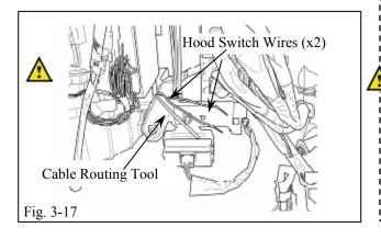
(t) Remove the electrical tape and Cable Wire Routing Tool. (Fig. 3-17)
