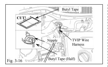
(s) Using ½ piece of Butyl Tape seal the Grommet nipple and Hood Switch Harness. (Fig. 3-16)
