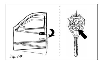
(m) Open the driver's door. Using the remote control, press the Lock button twice within 2 seconds, then press and hold the lock button for four (4) seconds. (Fig. 8-9)
