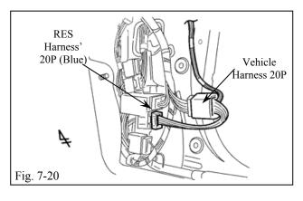
(y) Plug in the V4 Harness' BLUE 20P Connectors between the Vehicle harness' BLUE 20P connector and the Connector block. (Fig. 7-20)
