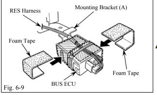
(k) Attach 2 pieces of Foam Tape to the BUS ECU as shown. (Fig. 6-9)
