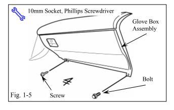
(f) Remove 1 Screw and 1 Bolt from the Glove box assembly. (Fig. 1-5)
