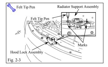
(c) Using a Felt Tip Pen, mark the Radiator support assembly and Hood lock assembly as shown. (Fig. 2-3)
