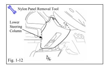
(n) Remove the Lower steering column cover. (Fig. 1-12)
