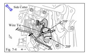
(e) Secure the white 20P Connectors to the Vehicle Harness with 1 Wire Tie. (Fig. 7-4)
