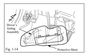
(p) Wrap the Airbag assembly in a Blanket and place it on the V4 Kit Box. (Fig. 1-14)
