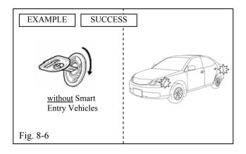
(i) Start the engine; after counting 10 seconds stop the engine. The hazard lights flash once. Registration completed. (Fig. 8-6)
