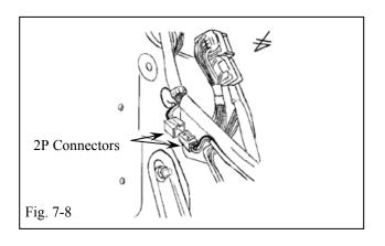
(i) Plug in the V4 Harness' White 2P Connector to the Vehicle Harness' White 2P Connector.(Fig. 7-7)
