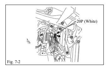
(b) Locate and disconnect the White 20P Connector from the Connector Block in the upper right area of the Glove Box. (Fig. 7-2)
