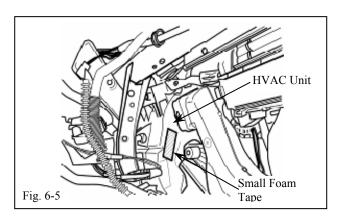
(f) Apply 1 piece of Foam Tape to the HVAC Center Duct. (Fig. 6-5)
