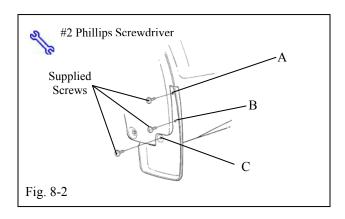
(b) While holding mudguard up and into body panel install supplied screws in locationsA, B and C. (Fig. 8-2).
