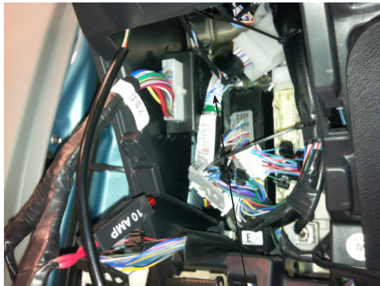
Mount control module to the left of this factory harness
