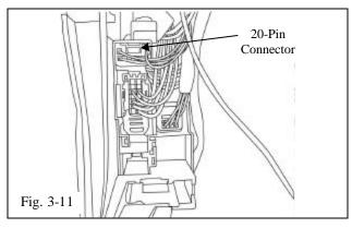
(k) Remove 20-pin connector from junction block. (Fig. 3-11)
