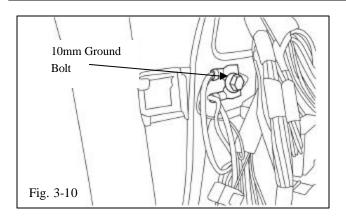
(j) Connect ring terminal from EC mirror harness to 10 mm ground bolt in cowl area.(Fig. 3-10)
