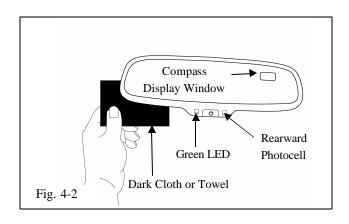
(4) Remove the cover from the forward-looking light sensor and the mirror will begin to clear.
