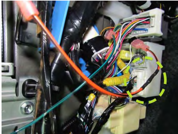
Picture 15: diode adapter circled in yellow
