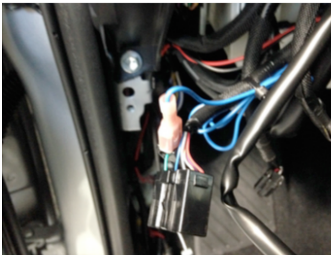
Picture 9: DRL blue wire to connector D35, pin1 (green wire)
