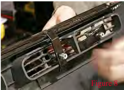
Rotate the brackets sideways and place billet grille into opening and center. Reaching on the backside of the bumper rotate the brackets around so that they catch the top of metal rail and bottom of plastic bumper opening as shown.
