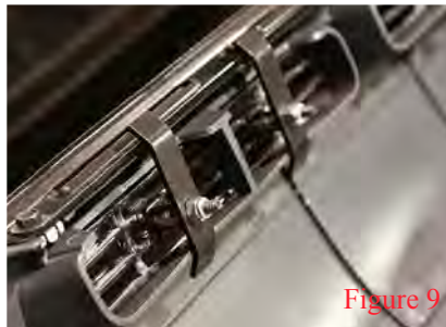
Tighten bolts using an allen wrench and ratchet to fasten.
