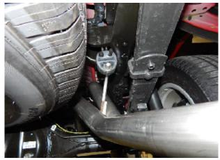
8. Place the hanger into the rubber isolator, fig.  $8\,$
