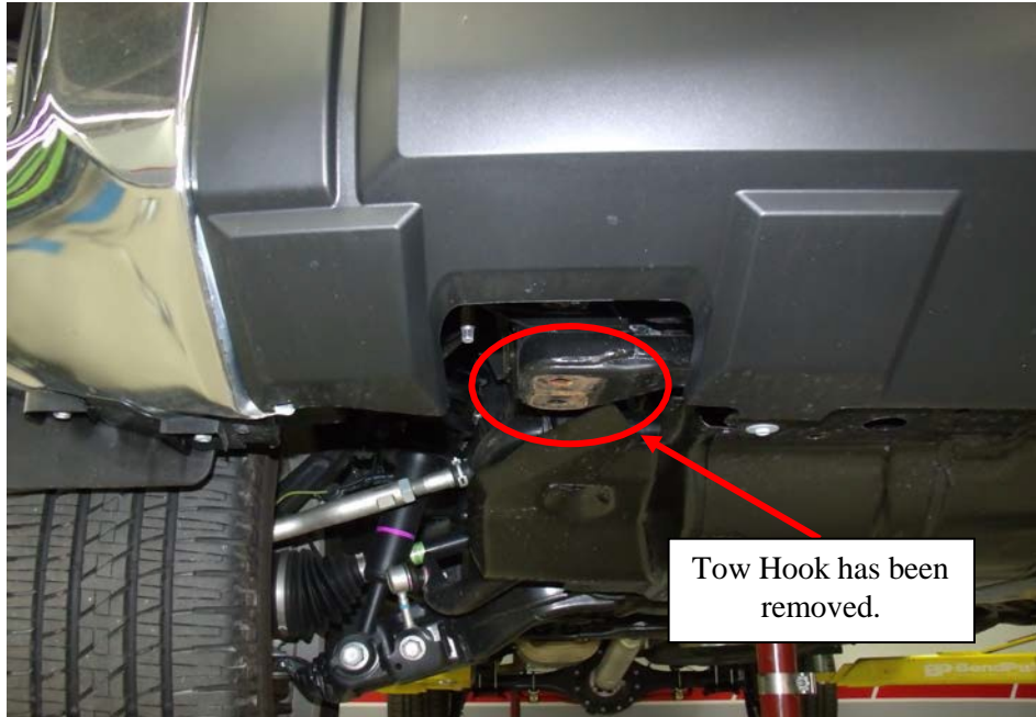
Figure – 5 – View of Passenger Side with Tow Hook Removed
