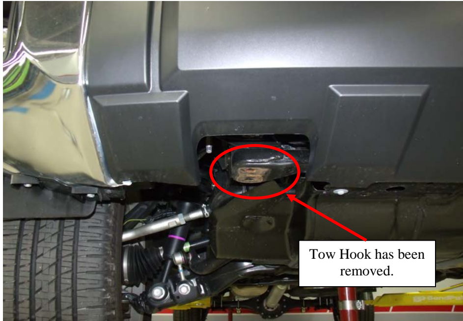
Figure – 4 – View of Passenger Side with Tow Hook Removed
