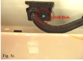
Tailgate side of harness with bottom marked to drill hole.
