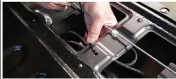
**Step 7:** Connect the Delphi end of the long wire harness to the Delphi end of the short harness. Secure the long wire harness under the truck bed maintaining easy access to the Delphi plug for tailgate removal. Also make sure the tailgate can be open and closed without pinching any part of the connector or the wire.
