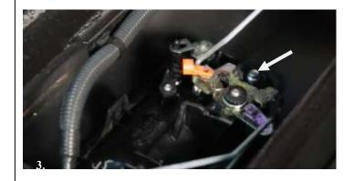
**Step 4:** Mount the power lock inside the tailgate to the passenger side of the handle. One hole in the bracket will align with the mounting bolt removed in the last step. The other hole will straddle a plastic post on the handle (see arrow). Insert the handle mounting bolt into the hole and tighten.
