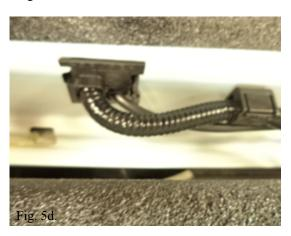
Tailgate side of harness with clip installed and harness routed.
