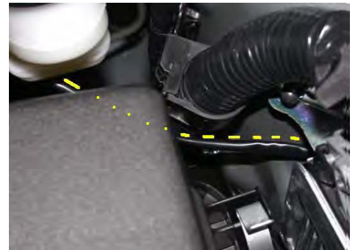
Picture 1C: Wire tie to the ECU harness
