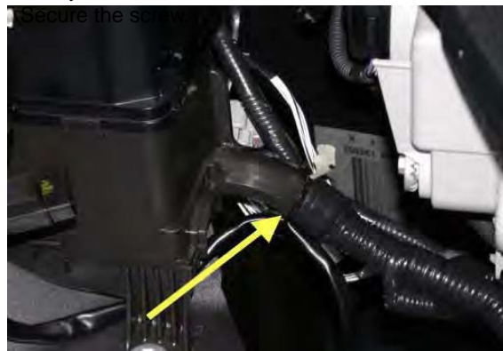
Picture 1A: Remove screw of the base of fuse box. Gently, lift the base and slide in the wire harness.
