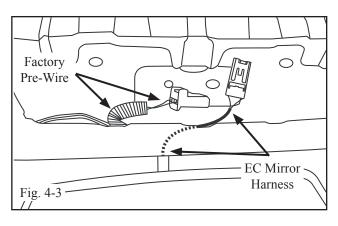
(c) Route EC mirror harness between vehicle roof and headliner into the overhead cavity. (Fig. 4-3)
