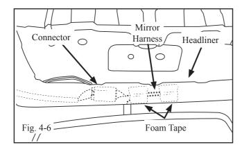
(f) Using two (2) pieces of foam tape, secure the remaining EC wire harness and factory pre-wire connector in overhead location as shown. (Fig. 4-6)
