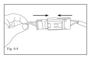
(d) Plug factory pre-wire 5-pin connector into the 5-pin EC mirror harness connector. (Fig. 4-4)
