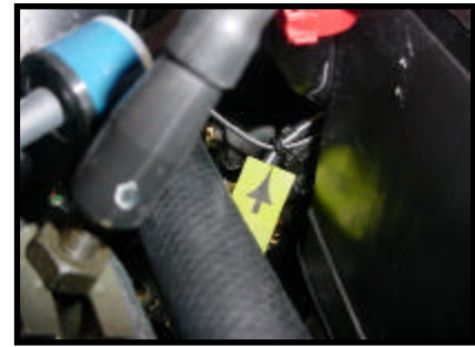
Wire tie on harness between battery and throttle.
