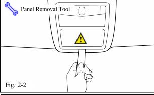
(b) With a panel removal tool, carefully remove the overhead dome light assembly. (Fig. 2-2)
