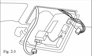
(c) Disconnect all connectors from overhead dome light assembly. (Fig. 2-3)
