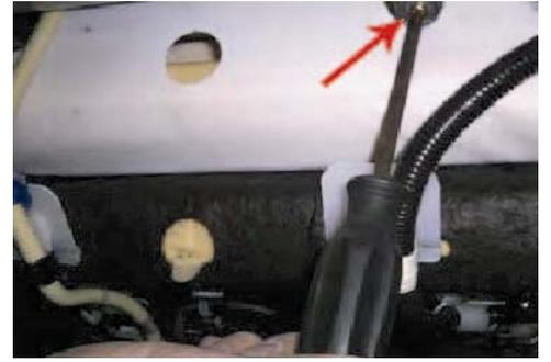
➡ 3. Pull out lower part of seat back to remove 2 mounting tabs. (Fig. H3)
