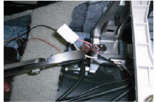
➔ 2. Attach the black wire from the control box to the T-tap on the white with black stripe wire (PIN#1) and the red wire from the control box to the T-tap on the red wire (PIN#2). (Fig. F2)
