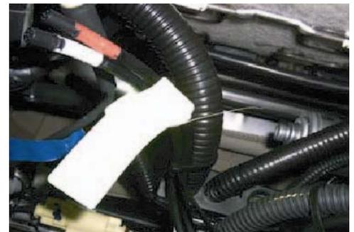
➔ 3. Bundle any excess wire using (1) wire tie and tuck under carpet. (Fig. E3)
