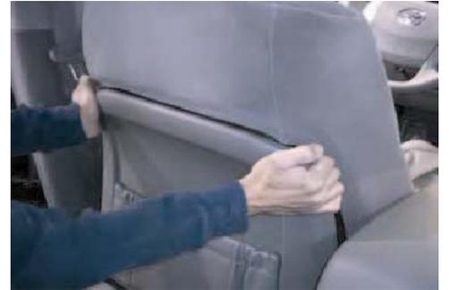
➡ 5. Lift out J-snaps to remove flap. (Fig. H5)
