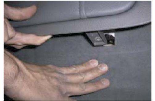
➡ 4. Push down on seat back to remove. (Fig. H4)
