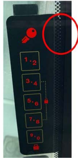
E: Light Leakage
