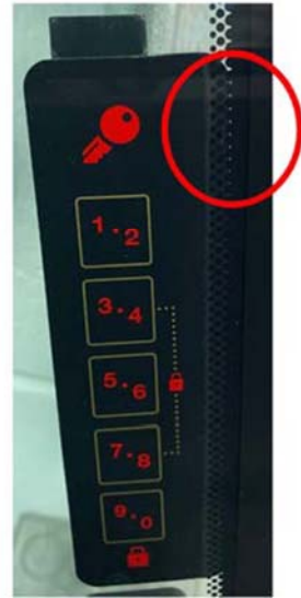
E: Light Leakage
