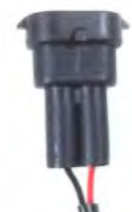
Picture 7A: Showing Fog light terminal connected.
