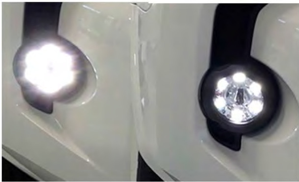
Left: showing LED Fog Light "ON" Right: Showing DRL "ON"
