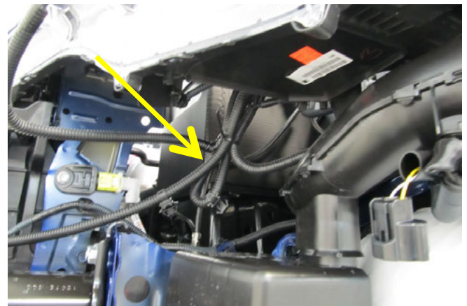
Picture 25: Driver side head-lamp: showing securing excess wires
