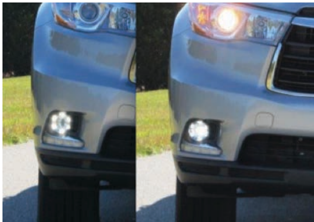
Right: showing LED Fog Light "ON" Left: Showing DRL "ON"
