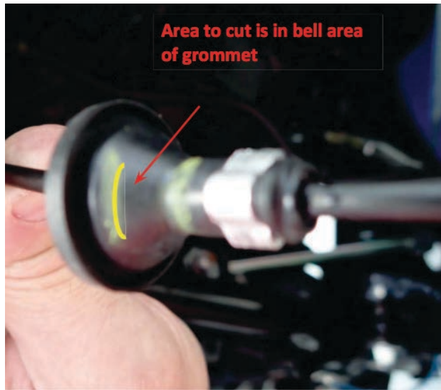
Picture 15C: Showing where to cut the grommet
