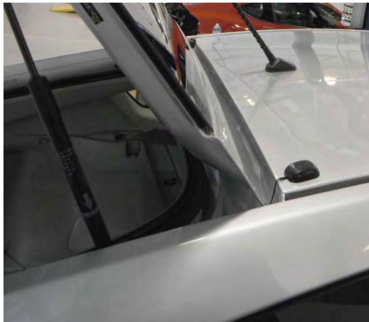
3. Secure the XM antenna cable to the body structure with provided foam tape.
