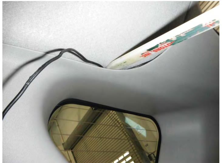
7. Partially remove the passenger's rear door pinchweld gasket.
