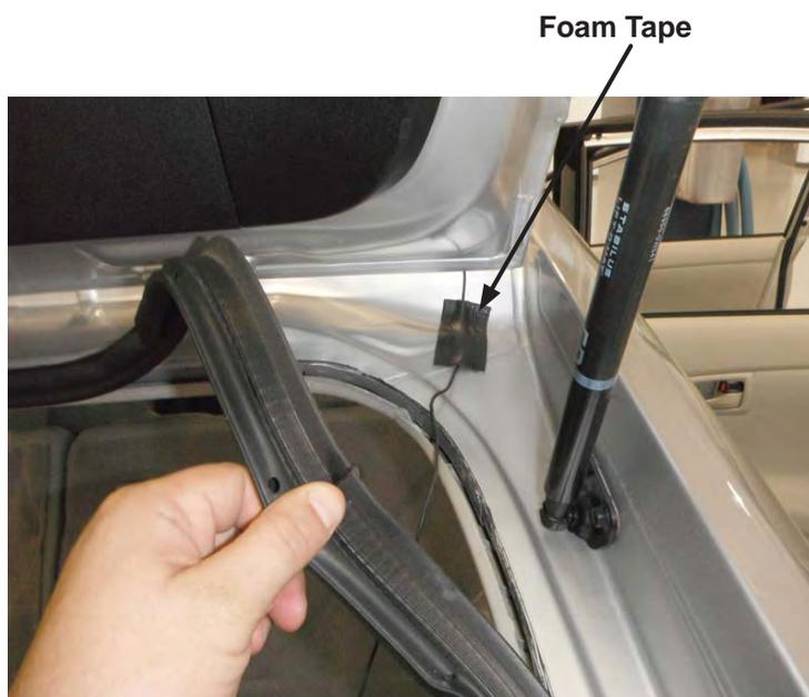
5. Reinstall the pinchweld gasket.
